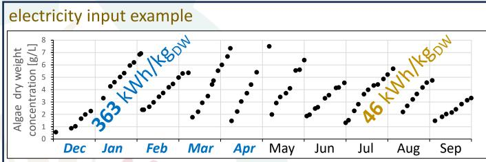
Growth of phototrophic microalgae in a 1500 Liter photobioreactor under sunlight *plus seasonal addition of electric light*. Direct electricity input excluding heating is compared
